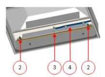
Figure 19: Removing the Sealing Bar (Metal Lid)
