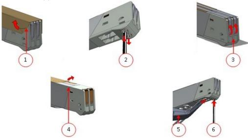
Figure 20: Replacing the Sealing Wire
