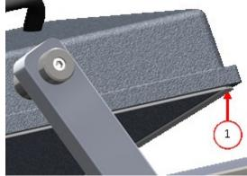
Replace the lid gasket if damaged or as specified in *Maintenance Schedule* on page 38.
