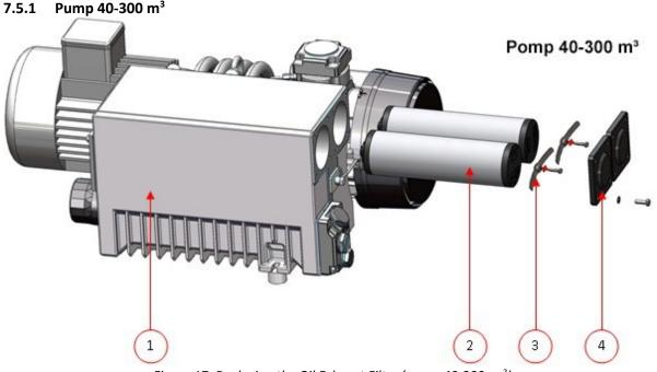
Figure 17: Replacing the Oil Exhaust Filter (pump 40-300 m<sup>3</sup>)
