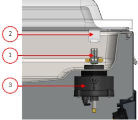
Figure 2: Overview of the Sealing System (Including Sealing Cylinder)
