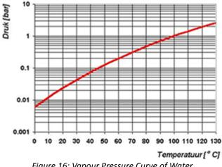
Figure 16: Vapour Pressure Curve of Water
