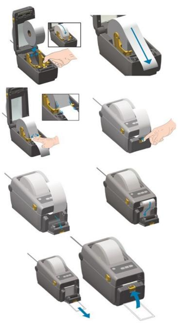
Figuur 23: Replacing the Printer Roll
