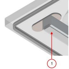
Figure 21: Replacing the Silicone Rubber of the Silicone Holders
